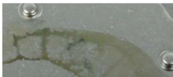
Fig. 2.1, Magnet surface with cured adhesive
